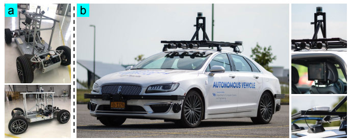
Figure 4: AD vehicles for the system-driven evaluation platform: (a) A real-vehicle sized chassis with L4 AD sensors and closed-loop control; (b) A L4 AD vehicle built upon Lincoln MKZ. Both are equipped with L4 AD-grade sensors such as LiDARs, cameras, RADARs, GPS, and IMU. Detailed specifications are on our project website https://sites.google.com/view/cav-sec/pass [25].
