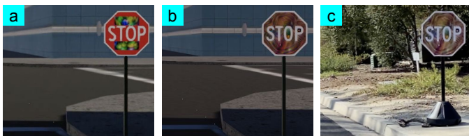
Figure 5: Reproduced semantic AD AI attacks on STOP sign hiding: (a) RP2 [18] in simulator, (b) SS [37] in simulator, and (c) SS [37] in physical world.
